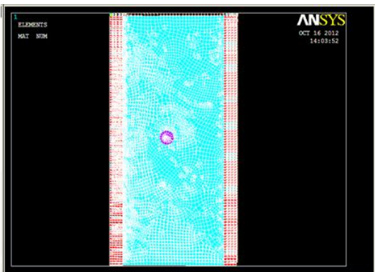
Fig.5 2 D model with 3 different areas ground, anomaly and free space inside slotted parallel plate transmission line.
