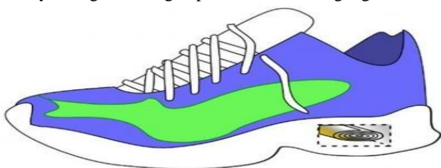
Fig.5.Piezoelectric crystals installed in shoes.
