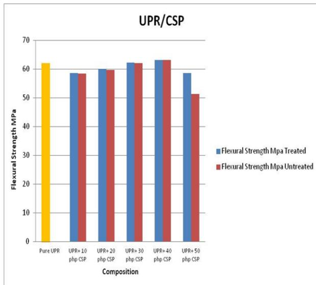
Fig. 5 The effect of filler content on the flexural strength of UPR/CSP composites
