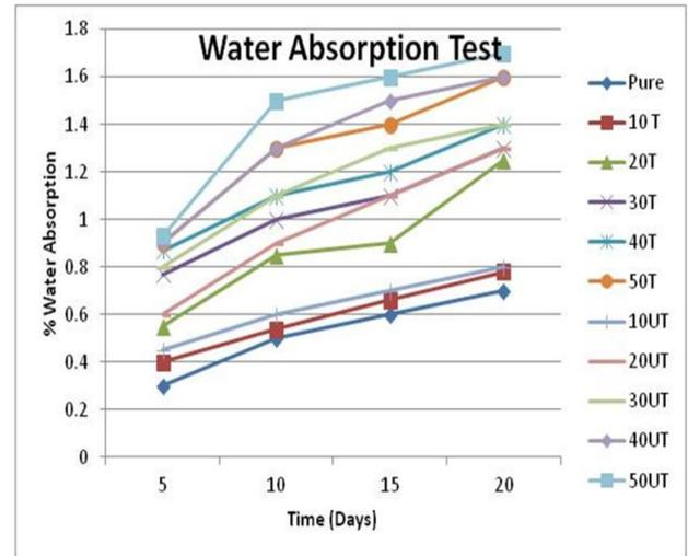
Fig. 6 Percentage of Water absorption versus Time on UPR/CSP Composites.
