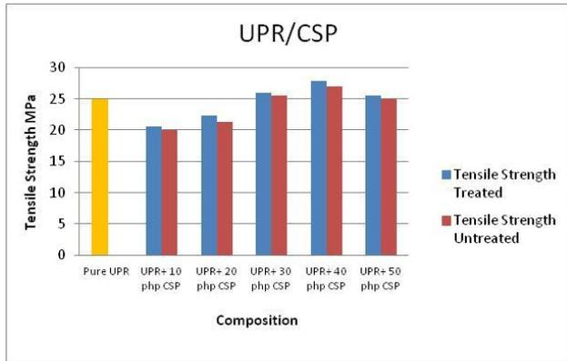
Fig. 4 The effect of filler content on the tensile Strength of UPR/CSP composites
