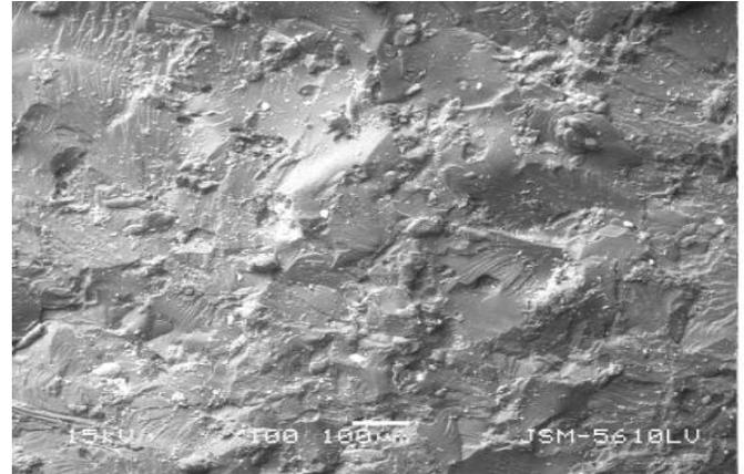
Fig. 2 SEM micrograph of tensile fracture surface of UPR/CSP composites (30% treated) at magnification of 100X.
