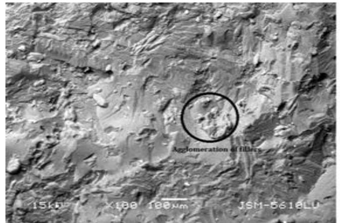
Fig. 3 SEM micrograph of tensile fracture surface of UPR/CSP composites (30% untreated) at magnification of 100X.
