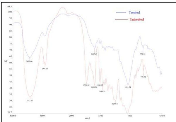
Fig. 1 FTIR Spectrum for treated and untreated CSP
