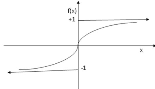
Figure-7 Tan Sigmoidal (Bipolar) Activation Function
