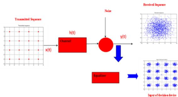
Figure 2 Channel equalization
