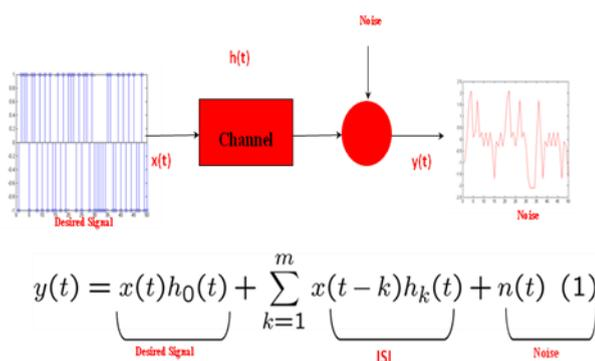
Figure 1 Communication Channel
