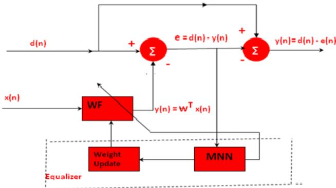
Figure-3 Channel Equalizer Using WF
