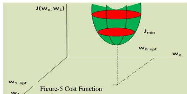
With the cross-correlation and autocorrelation as constants, this cost function is clearly a quadratic function in  $w_0$  and  $w_1$ . The minimum is at the bottom of the “bowl.” The derivatives of the cost function with respect to the two weights are
