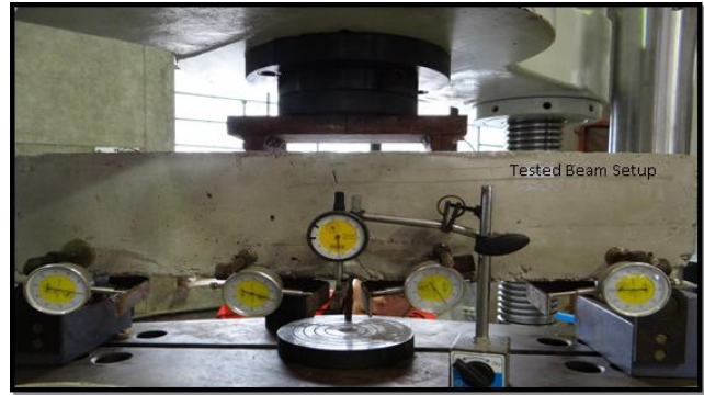
Figure (3) Loading frame and the specimen setup.
