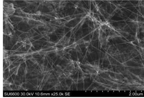
Figure 8: SEM image of the cathode cooled naturally in inert environment after 30 s of arcing.
