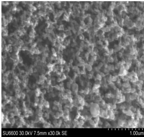
Figure 6: SEM image of vein graphite cathode after 10 s arcing at 40 A.
