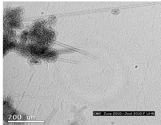
Figure 9: HRTEM image showing SWCNT produced.
