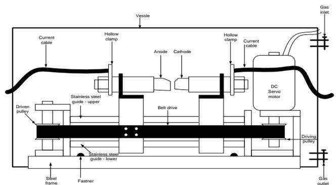
Figure 1: Block diagram of the apparatus used in the laboratory for CNT production
