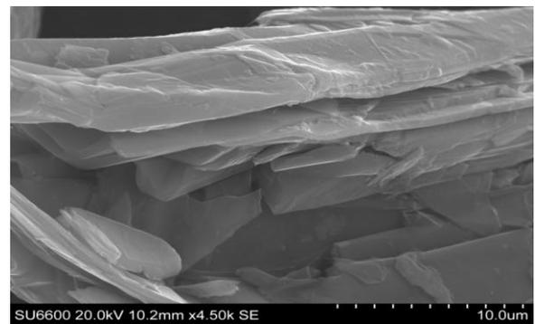
Figure 4: SEM image of vein graphite obtained from Sri Lanka used for CNT production
