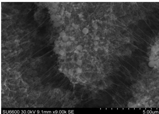
Figure 7: SEM image of the cathode cooled in inert atmosphere after 25 s of arcing.
