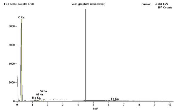
Figure 5: Energy dispersive X-ray analysis plot of vein graphite
