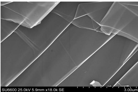
Figure 2: SEM image of flake graphite obtained from Sri Lanka
