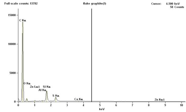
Figure 3: Energy dispersive X-ray analysis plot of flake graphite
