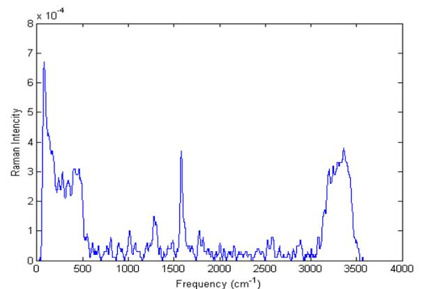
Figure 10: Raman spectroscopy results of the CNT sample
