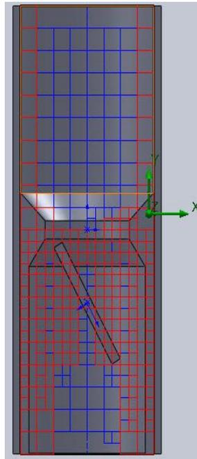
Figure 3: Meshed Structure of a Carburettor.
