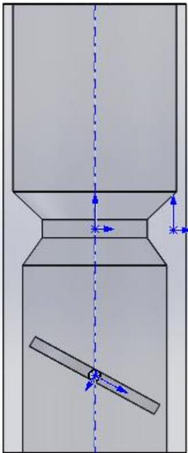
Figure 2: Model of a simple Carburettor
