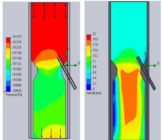
Figure 9(a): Pressure contour for 35 degree variation. Figure 9(b): Velocity contour for 35 degree variation.
