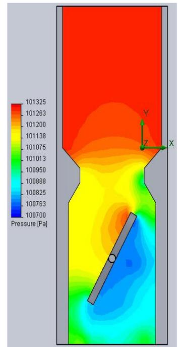
Figure 5: 60 Degrees Throttle Plate Angle.
