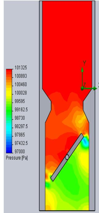
Figure 4: 45 Degrees Throttle Plate Angle.
