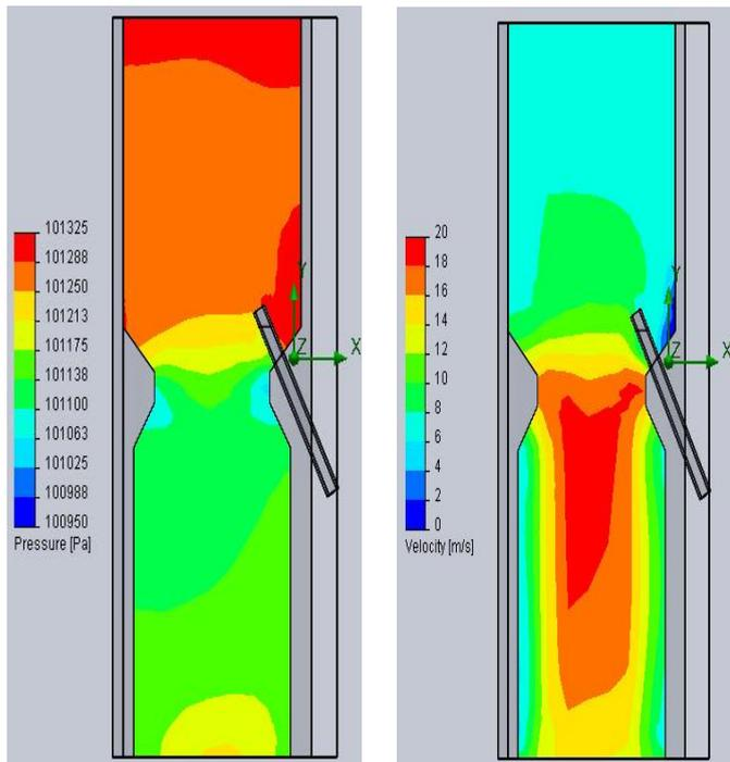
Figure 8(a): Pressure contour for 30 degree variation. Figure 8(b): Velocity contour for 30 degree variation.
