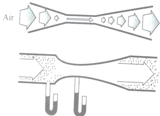
Figure 1: Operation of Venturi in a Carburettor
