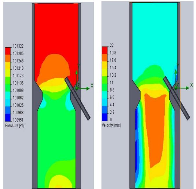
Figure 10(a): Pressure contour for 40 degree variation. Figure 10(b): Velocity contour for 40 degree variation.
