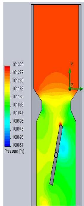
Figure 6: 75 Degrees Throttle Plate Angle.
