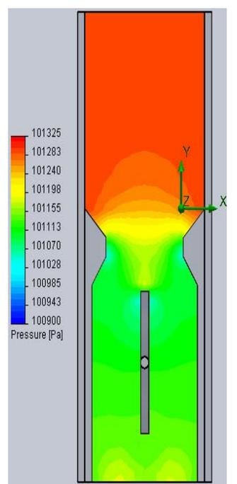
Figure 7: 90 Degrees Throttle Plate Angle.
