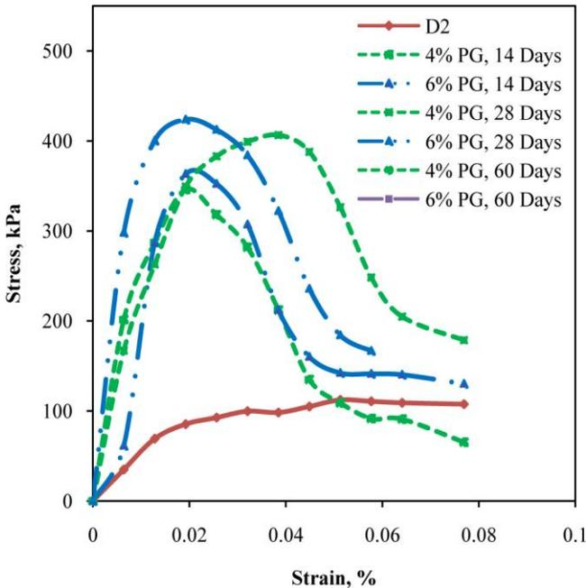
Figure - 2. Stress-strain curves from the unconfined compression test for soils mixed with different percentages PG and FA.
