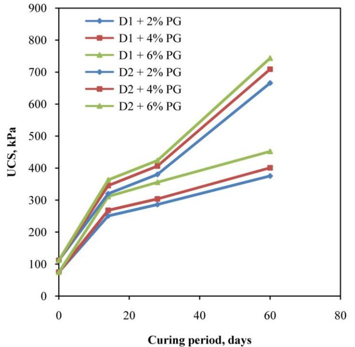
Figure - 3 . Strength development in treated clay samples for different curing periods
