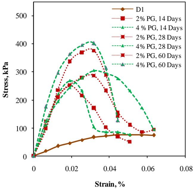
Figure - 1. Stress-strain curves from the unconfined compression test for soils mixed with different percentages PG and 5% of FA.
