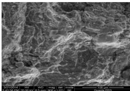
(d). D1 Soil Treated with 4% PG + 5% FA at 14 days curing period
