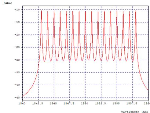
Fig.6 Spectrum of Combiner output for 16- Channel WDM Layout
