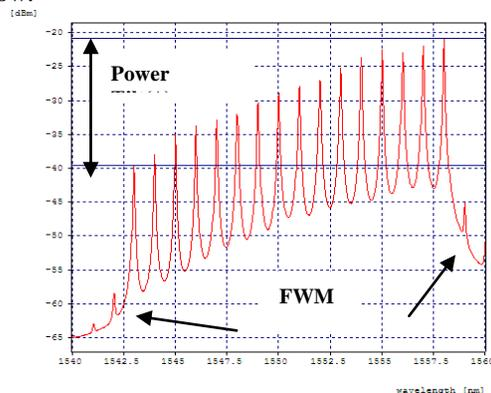
Fig.7 Fiber output spectrum for 16-channel WDM layout without Duobinary system
