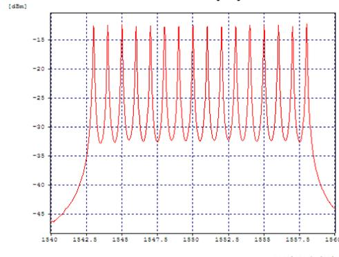
Fig.8 Fiber output spectrum for 16-Channel WDM layout with Duobinary system
