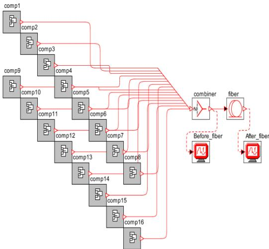
Fig.4 Optim layout for 16-channel WDM system with Duobinary Modulation
