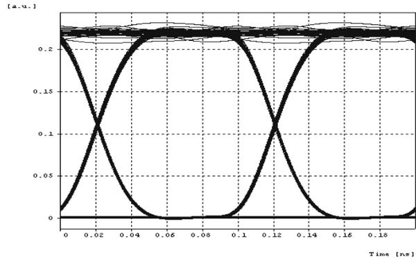
Fig 7 Eye diagram for 32 channel DWDM system with XPM compensation
