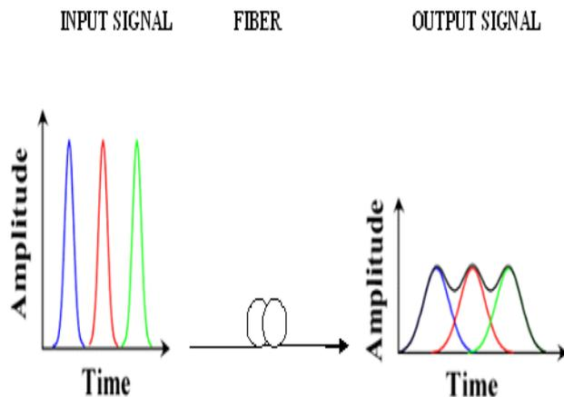
Fig 1 Pulse broadening for different length of the fiber
