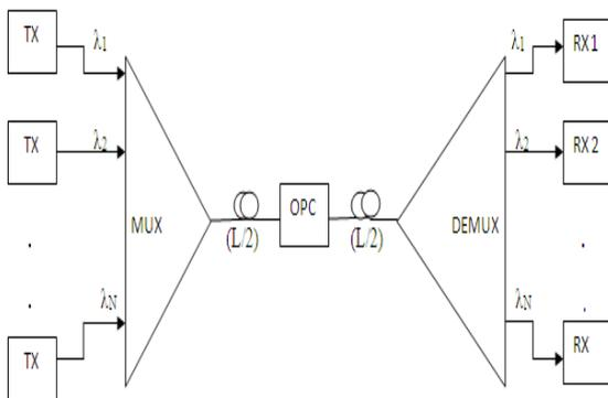
Fig 2 Block Diagram for XPM Compensation
