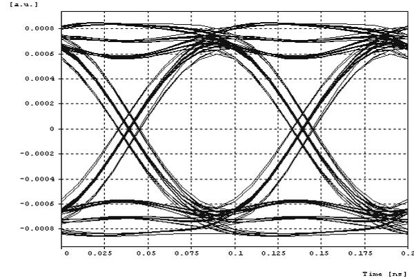
Fig 8 Eye diagram for 2 channel WDM system for DQPSK Modulation
