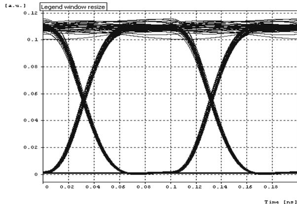
Fig 5 Eye diagram for 16 channel WDM System with XPM compensation
