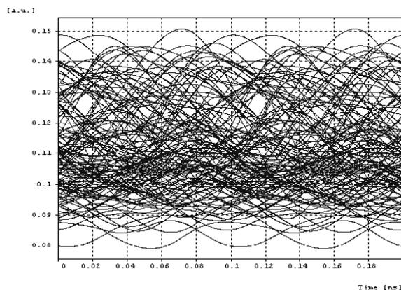
Fig 6 Eye diagram for 32 channel DWDM system without XPM compensation
