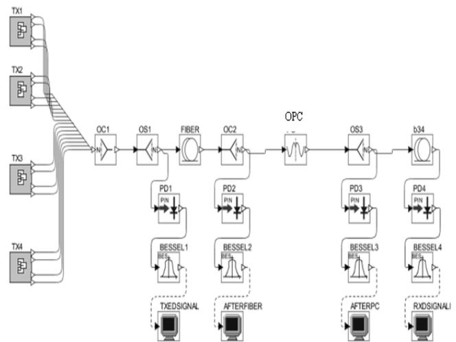
Fig 3 Optsim layout for 16 channel XPM compensation
