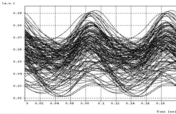
Fig 4 Eye diagram for 16 channel WDM System with XPM compensation
