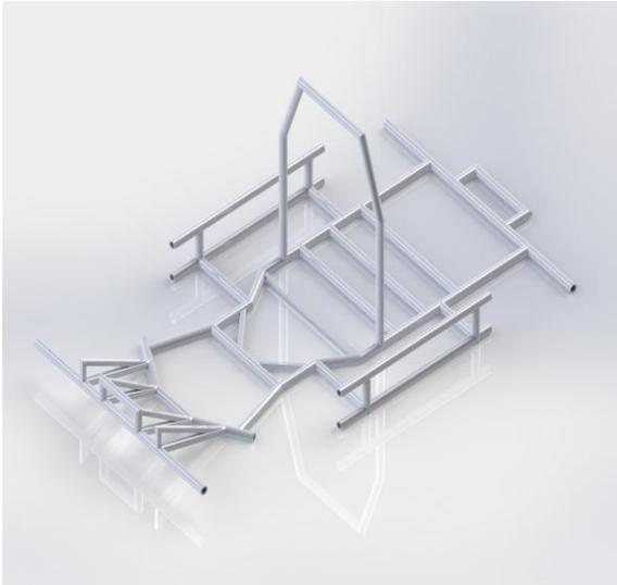
Figure no. 1 CAD model of Frame.
