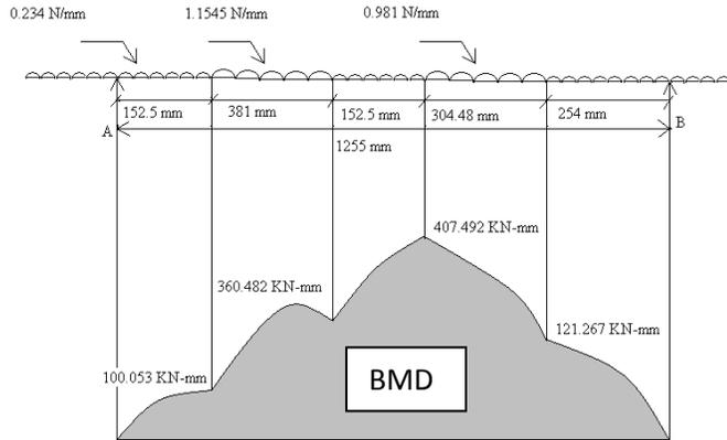
Figure no. 6 Beam with loading conditions and BMD.
