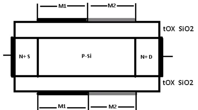
Figure 2. Dual Metal Double Gate MOSFET
