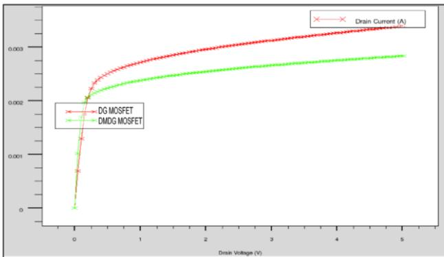
Figure 3. ID-VDS curve for DG MOSFET and DMDG MOSFET
