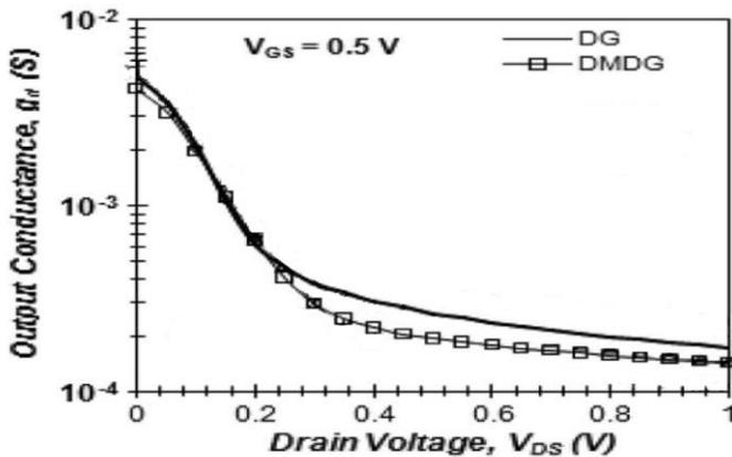
Figure 4. Output conductance- VDS curve comparison
