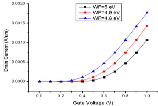
Fig. 2:  $I_d-V_{gs}$  Characteristics of JLVMOS at 45nm Technology.
