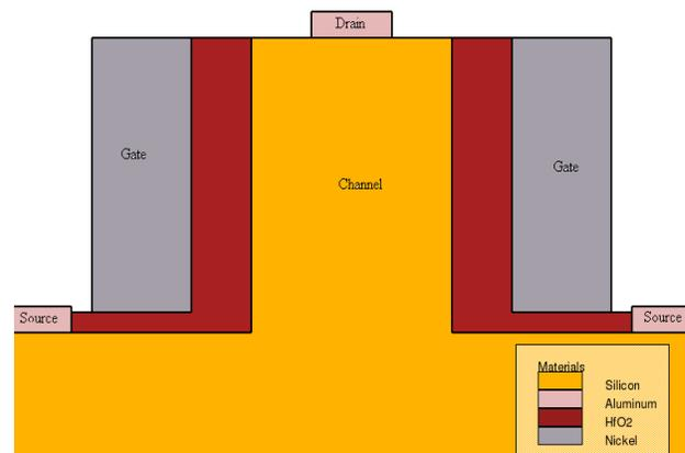
Fig.2: 2D Structure of Junctionless Vertical Double Gate MOSFET.
