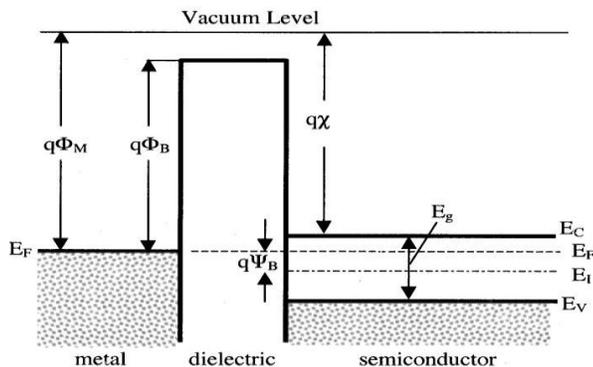
Fig.1: Energy-band diagrams of JLV MOS with metal gate electrode.
