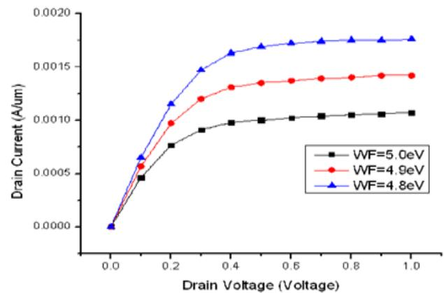
Fig.3:  $I_d-V_{ds}$  Characteristics of JLVMOS at different gate voltage of 45nm technology.
