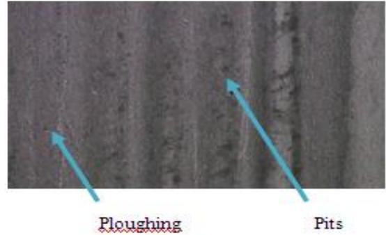
**Figure 2** Microstructure of Grade-A after Three Body Abrasive Test
