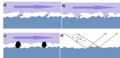
**Figure 1** a) adhesive wear, b)two-body abrasion, c) three-body abrasion and d) erosion
