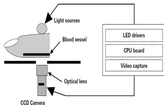
Fig 2 : Image capture using principle near infrared radiation
