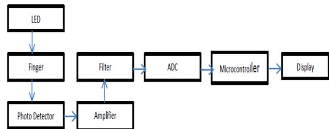
Fig 1 Pulse Oximeter Block diagram
