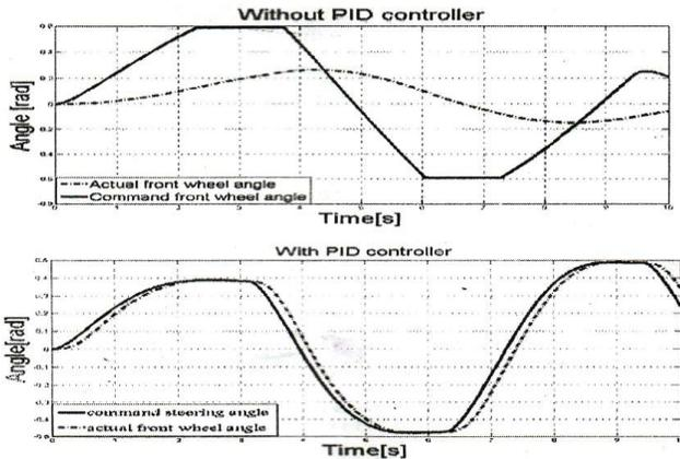
**Fig 3.2 Front Wheel Tracking Results**
