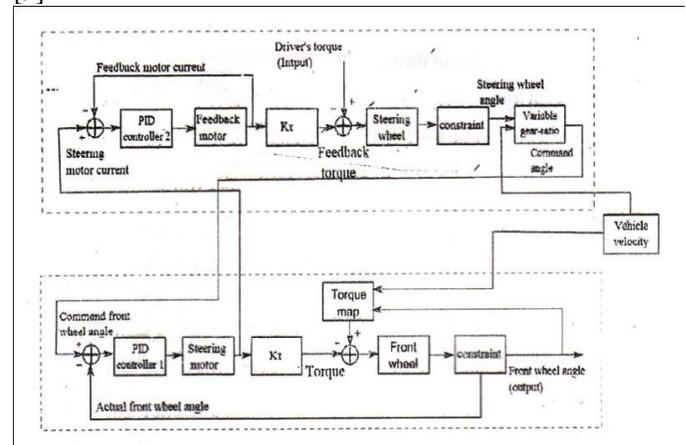
**Fig 1.1 Control System Model Design**
