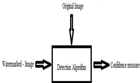
Figure 2: Watermark Extraction Process
