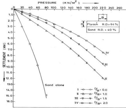
Fig.1 Pressure-Settlement for fly ash over sand for different relative densities
