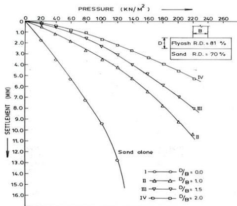
Fig.2 Pressure-Settlement for fly ash over sand for different relative densities
