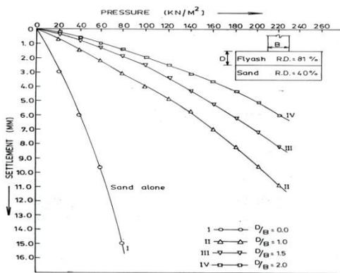
Fig.3 Pressure-Settlement for fly ash over sand for different relative densities
