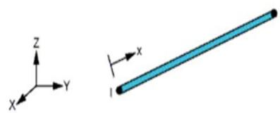
Figure3 - LINK8 Geometry
