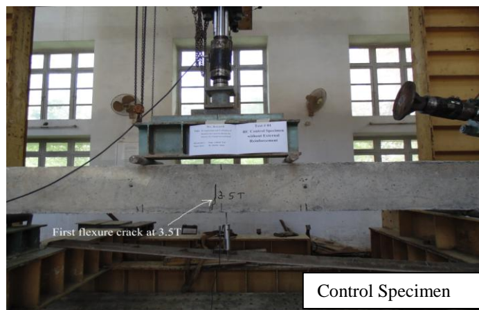
Figure: 5 Failure of Control Specimen BS1
