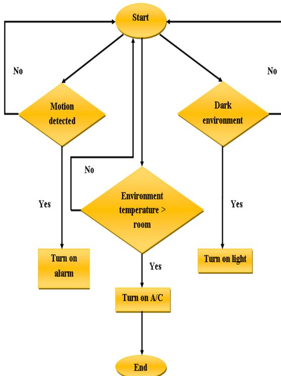
Figure 2 Flowchart of Hardware Mechanism
