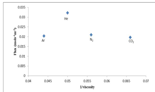
Fig. 4 Gas Flux ( $\text{molm}^{-2}\text{s}^{-1}$ ) against inverse viscosity ( $\text{Pas}^{-1}$ ) at 0.1 bar and at 413 K.
