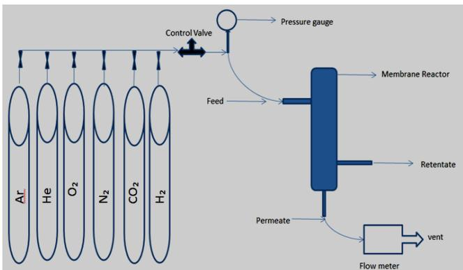
Fig. 2 Experimental setup for the gas permeation test
