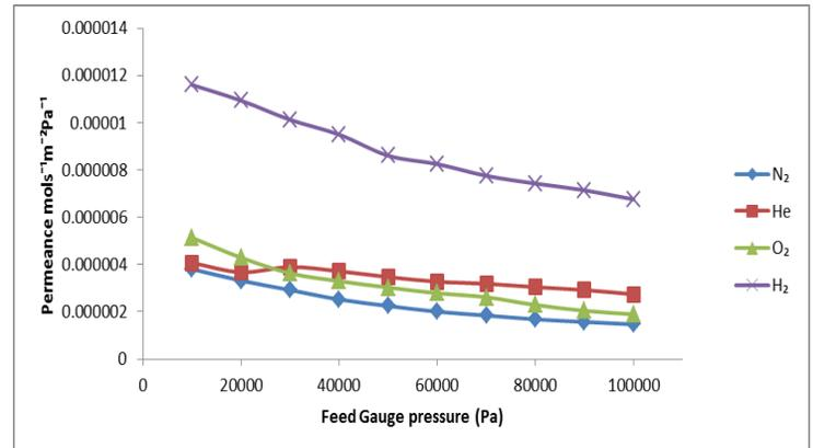
Fig. 6 Permeance (mols<sup>-1</sup>m<sup>-2</sup>Pa<sup>-1</sup>) against feed gauge pressure (Pa) at 298 K
