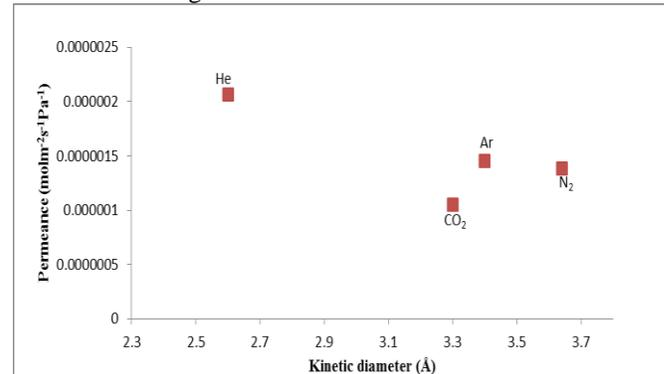
Fig. 3 Permeance ( $\text{molm}^{-2}\text{s}^{-1}\text{Pa}^{-1}$ ) against kinetic diameter (Å) at 0.4 bar and 413 K.
