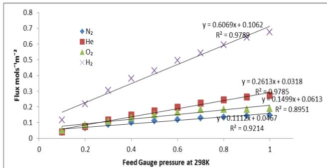
Fig. 5 Gas Flux (mols<sup>-1</sup>m<sup>-2</sup>) against feed gauge pressure (bar) at 298 K.
