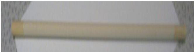
Fig. 1 Picture of the 15nm pore size commercial ceramic membrane.
