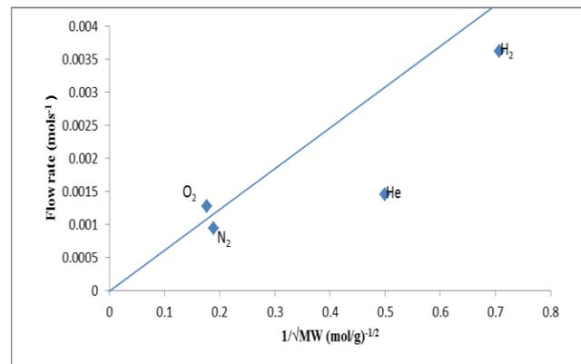
Fig. 7 Flow rate (mols<sup>-1</sup>) against Inverse square root of molecular weight (mol/g)<sup>-1/2</sup> at 0.5 bar and at 298 K.
