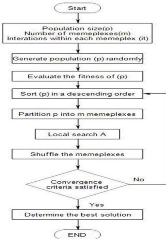
Chart(1). Shuffled frog leaping algorithm flowchart [vi].
