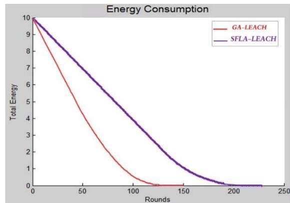
Figure (5). The network energy consumption in each round with  $E_0 = 0.1$
