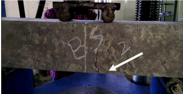
Fig 4: Initiation of failure pattern
