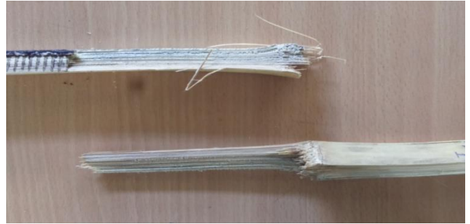
Fig 2: Failure of specimen due to axial load.
