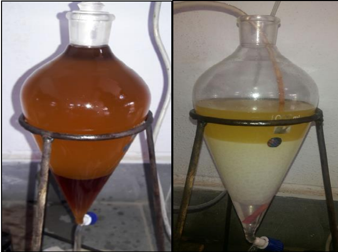
Fig. 4 Glycerin separation Fig. 5 Separation of soap
