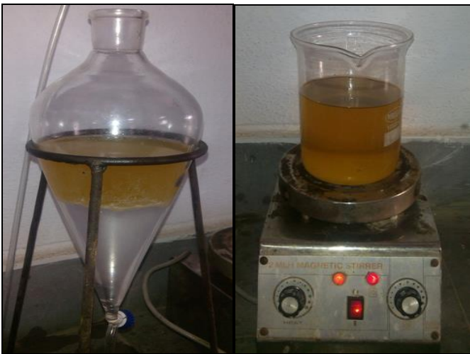
Fig. 6 Clear water in water washing Fig. 7 Biodiesel heating
